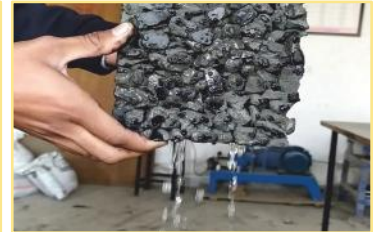
Permeable Concrete Pavement
